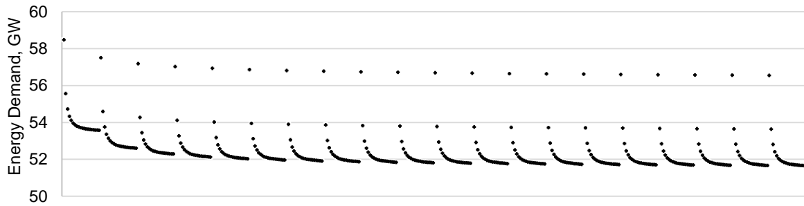
Figure 10 Overall annual energy demand calculated for development rises of 1 to 20 stories. Consecutive trends show energy demand of increasing rises of office development for each residential rise
