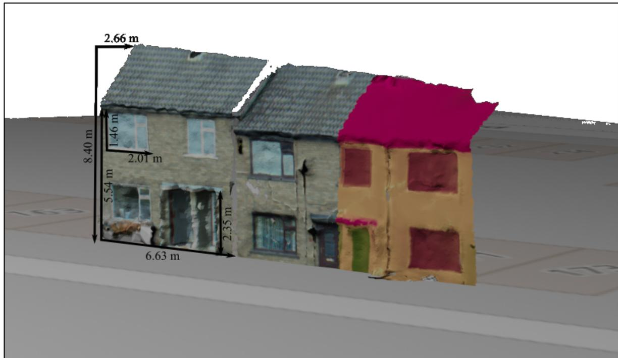
**Figure 3.** Examples of three reconstructed houses. Measurements overlaid on the left-most property show the dimensions of the facade, total structure, and a window and door. The central property shows the reconstructed facade with no annotation. The right-most property shows the results of labels projected onto the surface, which are used to measure the buildings.
